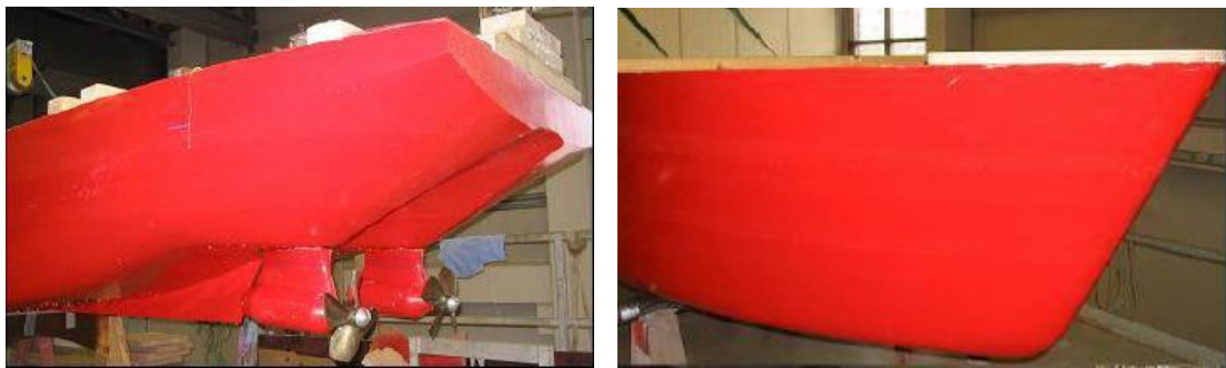
Fig. 9, Photographs of bow and stern of shuttle tanker of 1:28 self-propelled model ( courtesy of AARC )
