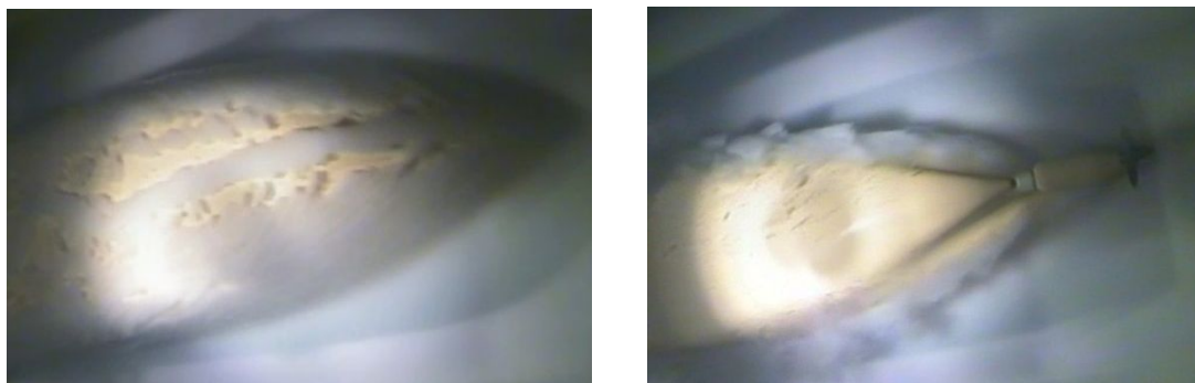
Fig. 8, Photographs from underneath a self propelled model in level ice showing fewer pieces of broken ice along the hull bottom due to the washing effect of the propeller wake (courtesy of Helsinki University of Technology)
